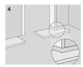
If possible, start to lay panels under the door jam and finish installing planks on a wall without a door jam. See "Working with Limited Clearance" section.
