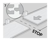
Lay panels close together on the floor.
