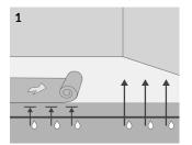
Install vapor barrier if subfloor is cement (6 mil polyethylene film).
