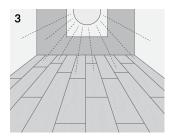
Install parallel to main light source. If no exterior light source, install parallel to longest wall.
