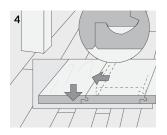
Slide panel into space horizontally and slot into profile. Use these modified planks under doorframes, radiators, cabinet fronts, etc. Use the pull bar to slide the planks where necessary.
