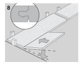
Rock and lock in half-length panel with rotating motion. Install the first and second row at the same time. This will help ensure end joints are perfectly square. Planks forced down without properly engaging the tongue into the groove can result in damage.
