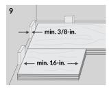
Observe 3/8" clearances for expansion and 16" minimum for smallest usable piece.
